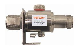
Ventev's Lightning Arrestor is a bi-directional gas discharge tube suppressor that features wide-band operation up to 7 GHz and is rated at IP67. Simply attach the lightning protector to an access point to help protect an entire network, outdoor antennas, and other wireless equipment from the build-up of static electricity. It is recommended to use 18 American Wire Gauge (AWG) ground wire.
